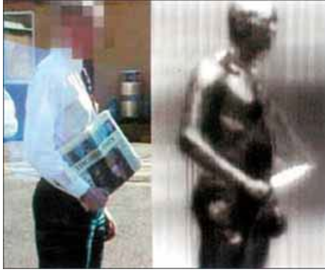
Figure 6. THz imaging of concealed weapon (Network, 2006)
